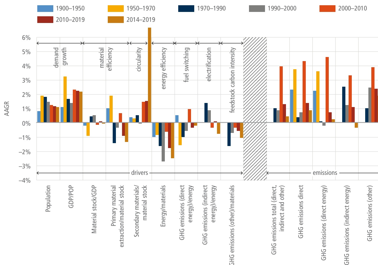
Figure 11.2 | Average annual growth rates of industrial sector GHG emissions and drivers (1900–2019). Before 1970, GHG emission (other) is limited to that from cement production. Waste emission is excluded. Primary material extraction excludes fuels and biomass. Presented factors correspond directly to Equation 11.1. Sources: population before 1950 and GDP before 1960: Maddison Project (2018); population from 1950 to 1970: UN (2015); population and GDP for 1960–2020: World Bank (2021); data on material stock, extraction, and use of secondary materials: Wiedenhofer et al. (2019); data on material extraction: UNEP and IRP (2020); industrial energy use for 1900–1970: IIASA (2018), for 1971–2019: IEA (2021b); data on industrial GHG emissions for 1900–1970: CDIAC (2017), for 1970–2019: data from Crippa et al. (2021) and Minx et al. (2021).
